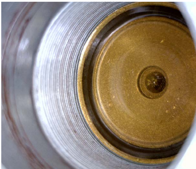
Body/O-Ring/Diaphragm - no significant areas of concern
