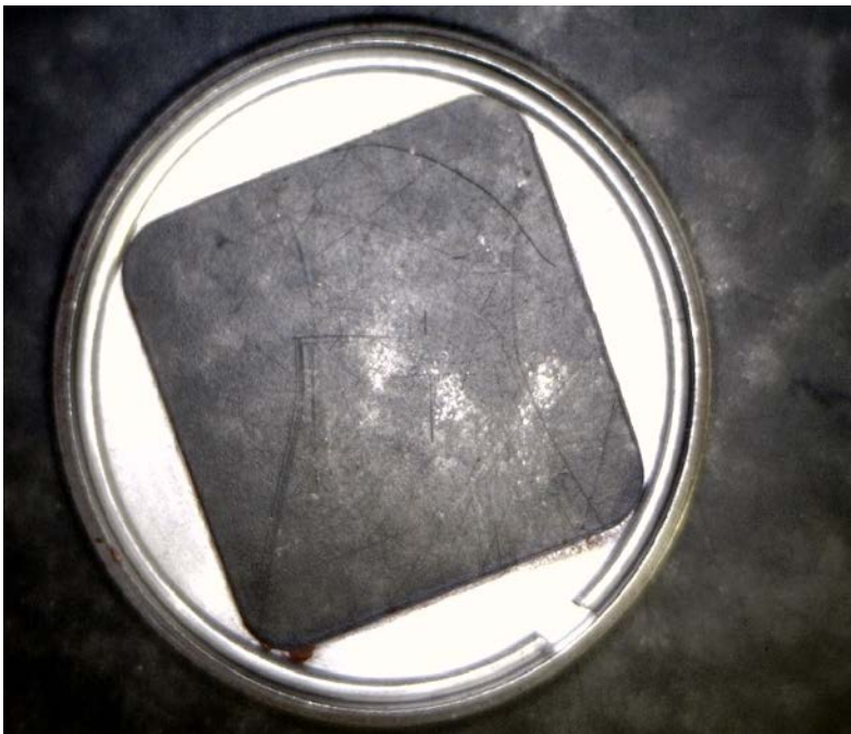
Retainer/Register Ring - Acceptable; good condition
