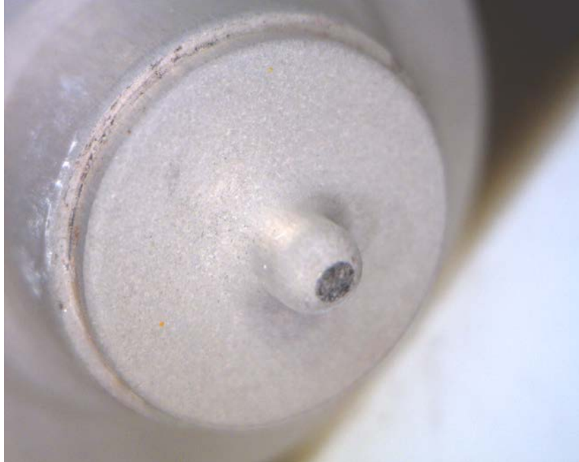
Pressure Plate - worn down to a flat (should be a full radius)
