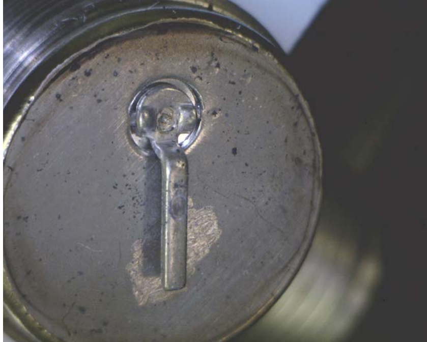
Switch Actuator Assembly - functional; minor wear on arm at point of pressure plate contact
