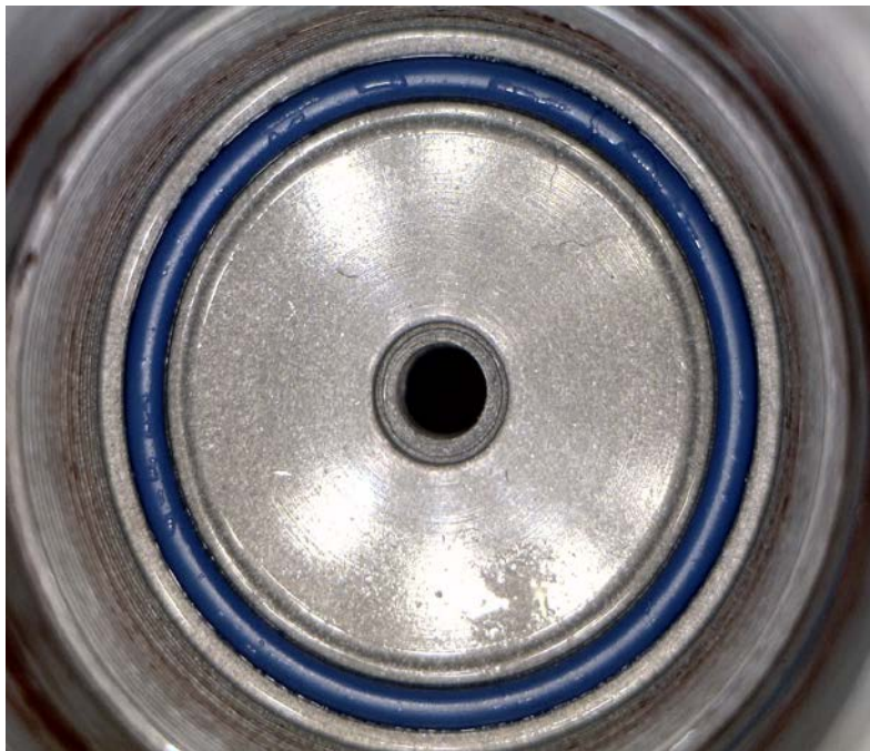
Body/O-Ring - some possible FOD; oily surface of body
