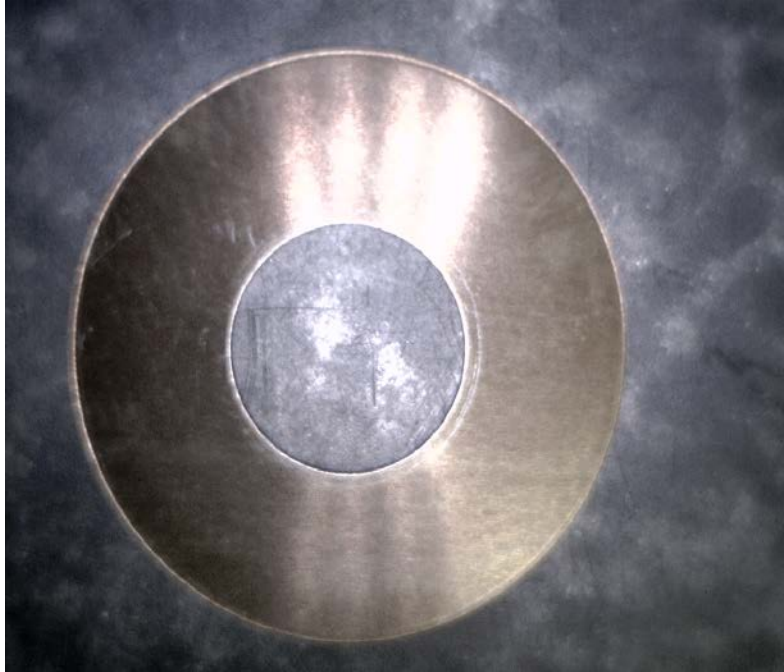
Disc Spring - Acceptable; minor signs of normal wear from cycling
