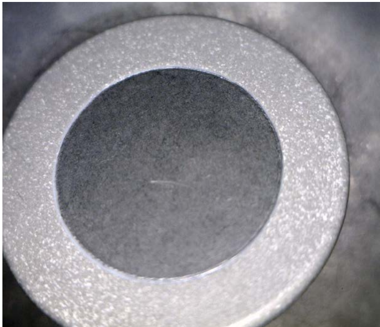
Pressure Plate/Plate - Acceptable; no signs of wear
