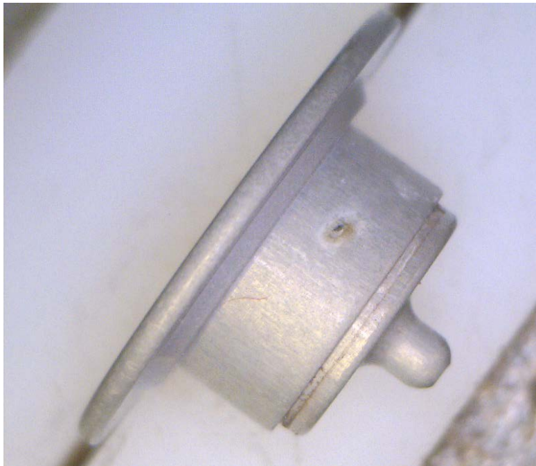
Pressure Plate - worn down to a flat (should be a full radius)
