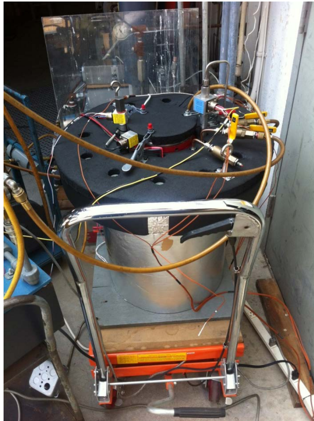
Figure 40: Explosion Proofness - Test Chamber
